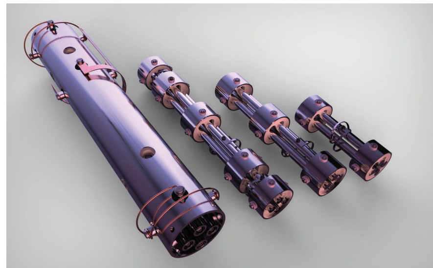
Figure 3: Quadrupole mass filters shown, from 20mm pole diameter to 6mm pole diameter offer mass range options up to 5000u. 200u mass range is typically used for most real time gas analysis applications.
