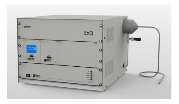
The inert, fast-response inlet system operates at up to 200°C with response times less than 300 milliseconds. The fully integrated system is now configurable both for benchtop and for rack-mounting operation, and is mountable as standard up to 2M from the sampling point.
