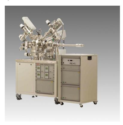
The fine-focus Hiden IG-20 gas-source ion gun generates both oxygen and noble gas ion beams with spot size down to 50 micron. The IG-5C ion gun, with the Hiden caesium surface ionisation source for analysis of electronegative species, has a spot size of just 20 micron. The EG-500 electron gun provides charge neutralisation of insulating surfaces.
