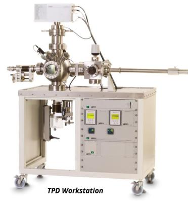
The quadrupole mass spectrometer, also with water-cooled jacket, is mounted with the acceptance aperture close to the sample surface for optimum capture of evolved gases, the 300 amu Hiden 3F PIC system featuring a fast digital detection system with 7-decade dynamic range for optimum quantification of evolved peak profiles. Sample temperature is merged directly with the TPDsoft control and acquisition program for combined presentation of multiple evolved species with temperature.
